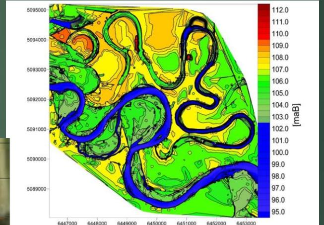
Figure 3.3. - Potentially water covered areas at the proposed 102.75 mAB water level
